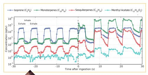
Human breath was monitored in real time at 3 Hz before and after the ingestion of a Ricola<sup>TM</sup> herb cough drop. Hundreds of compounds were present in the post-ingestion data, including monoterpenes, sesquiterpenes, and other compounds of herbal origin. A subset of detected compounds is shown in order to demonstrate the fast time response and broad dynamic range of the Vocus PTR-TOF.
