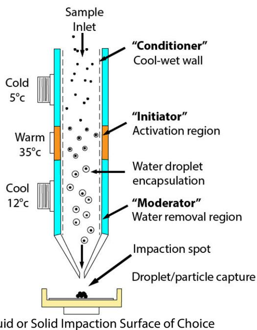
The Spot Sampler collector uses a patented, three-stage “moderated” condensational system to enlarge aerosol particles and then gently deposit them by inertial impaction.
