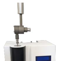
Inlet Cyclones can be used to select upper size of aerosol entering instrument
